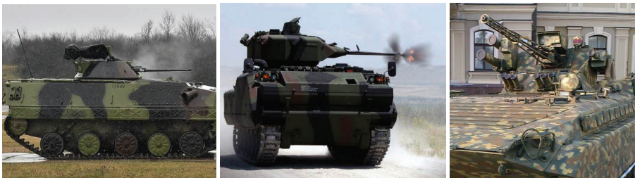
Figure 1: Light infantry fighting vehicles: “BVP M80A” with 20 mm autocannon, “FNSS ACV-15” with 25 mm autocannon and “BMP-1U Shkval” with 30 mm autocannon and 30 mm AGL [4-6]
